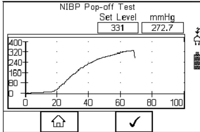
At the end of the test, the UNI-SIM will show the set-point of the protection valve (ie 331 mmHg)
