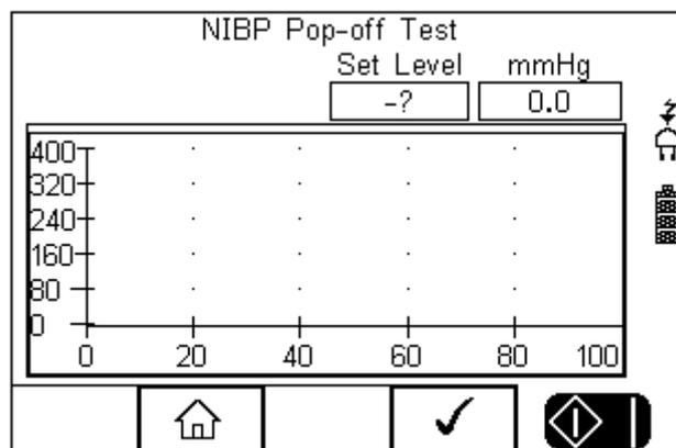
To initiate the test, press
