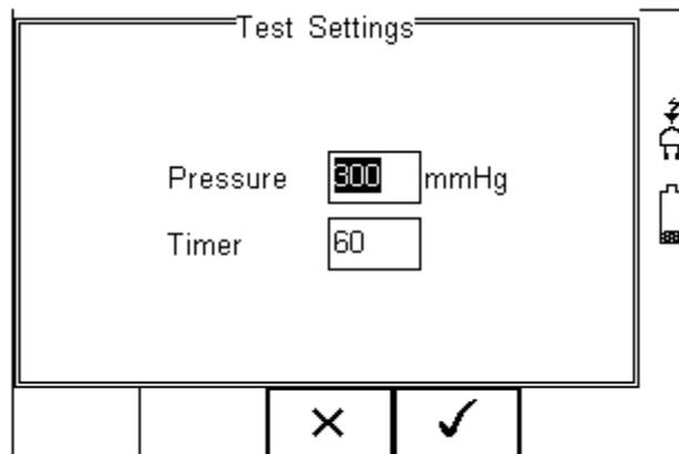
Highlight the required field using the up and down keys. To change the content use the keypad to enter the correct data. To Delete the field content, press the
