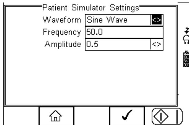
The preferred wave form and amplitudes can be selected by selecting the dropdown box (right arrow key) and use the up and down keys to select. The frequency can be entered manually.
