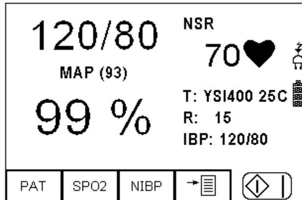
Alternatively, the user can choose between selecting a single or all of the simulation settings (ie NIBP (F3), SPO2 (F2) or PATient (F1) simulator) or entering the menu (F4) allowing for automatic testing, modifying the simulators default settings, viewing and downloading data and other user settings.
