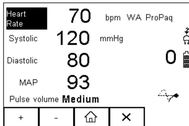
Using the Function keys (F1-F2), and up and down arrow keys, the highlighted field (change using arrow keys) can be changed using the “+” and “-“ function keys F1 and F2.
