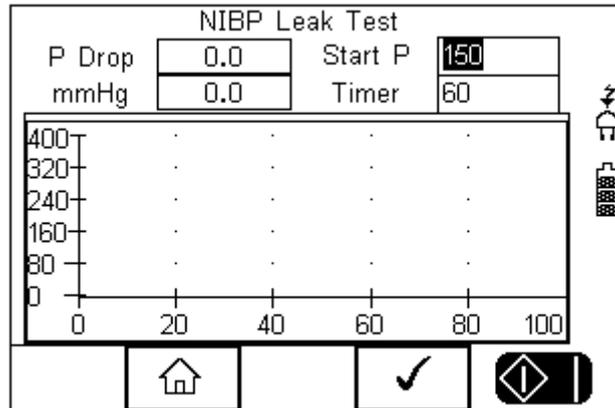
The UNI-SIM will inflate the system to around the set-point. Once the system is stabilised at the set pressure, the timer will count up for the set duration. This is highlighted below:
