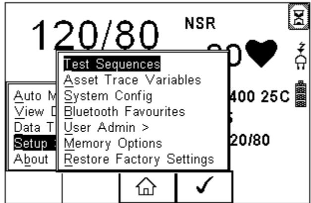
The following screen displays the list of default and customised tests available. Copied Test Sequences will appear in the list with an \*pre-fix.
