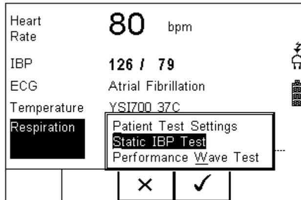
In the next screen, enter the required static pressure setting; The value entered is in mmHg and the UNI-SIM will simulate using an output of  $5\mu\text{V/V/mmHg}$ .
