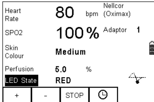
Whilst the simulation is being performed, the UNI-SIM can change settings. Use the arrow keys to scroll to the setting and use the “+” and “-“ keys to change the values.
