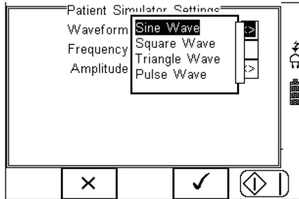
Confirm by pressing the
