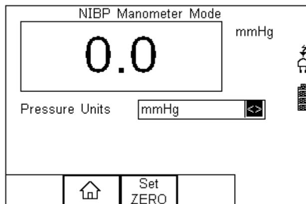
Ensure the manometer is set to zero by pressing the SET ZERO (F3) button) whilst the pressure connection at the UNI-SIM panel is open.
