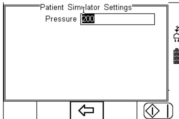
The simulation is continuously running whilst in this screen. When exiting this screen, the UNI-SIM will revert back to the systolic and diastolic settings, see 7.1.2)
